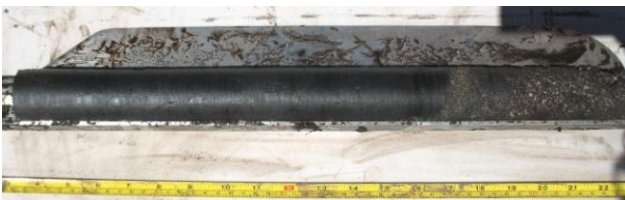
Figure 16h. Peaty silts under a gravel band, Boboyan Fen, ACT. Photo: Ben Keaney
